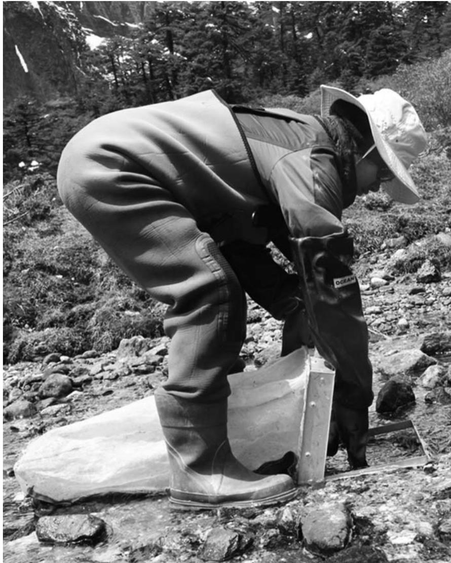
**Figure 2:** Sampling of stream benthic macro-invertebrates using hand net (frame of 25 cm and 25 cm) having 500  $\mu$ m mesh size in Langtang.
